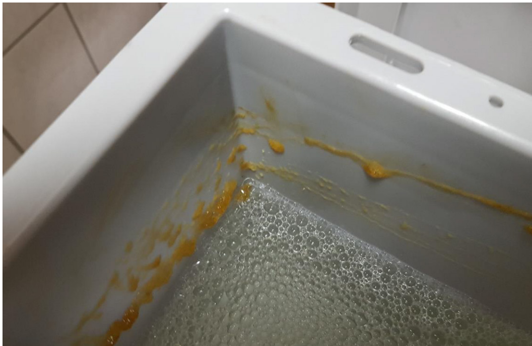
Figure 8: Grease residues on the inside of the tub after approx. 190 hours of operation with belt lubricant (water + 0.35% Lubricant)
