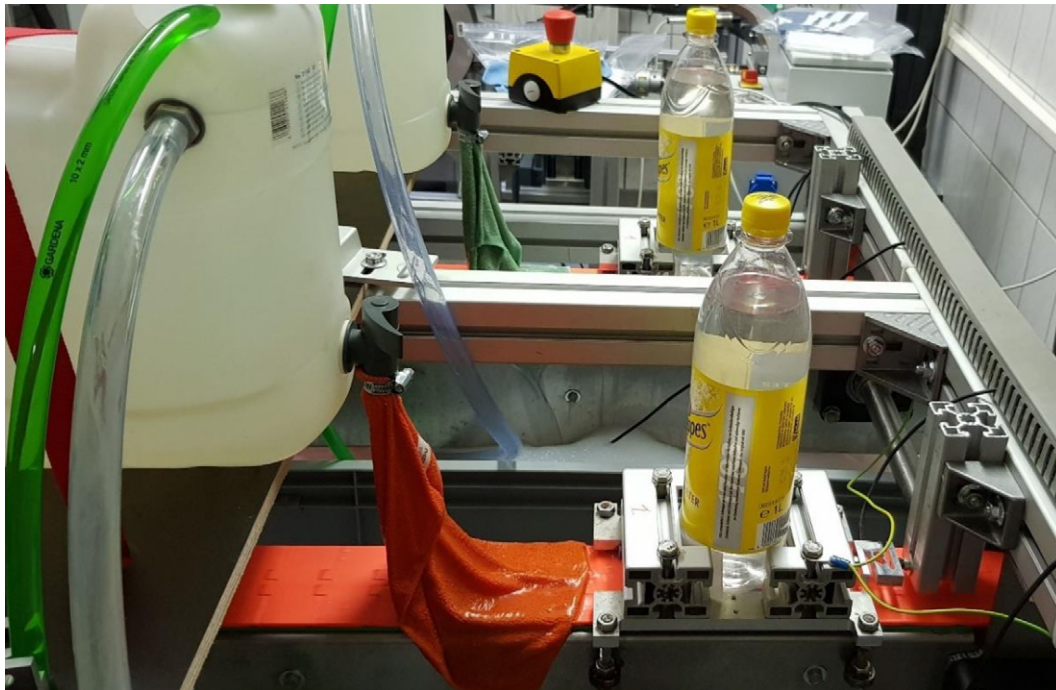
Figure 7: Continuous water or lubricant application via circulation pump.
