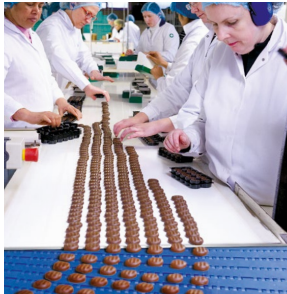
FDA ZERO CONTACT MODULAR BELT
